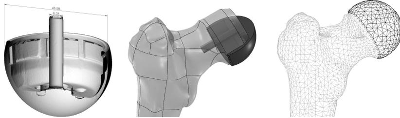
**Fig. 4.** Geometry of the cap-prosthesis, CAD model and generated FE model.
