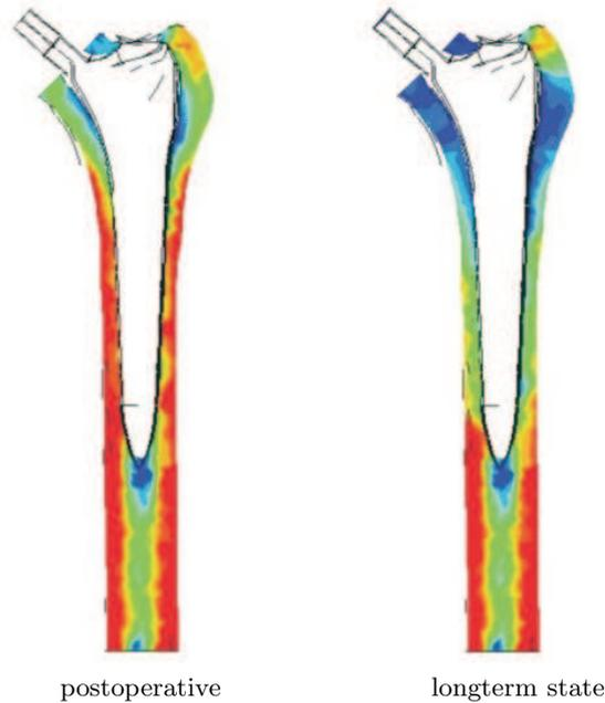
**Fig. 6.** Bone mass distribution computed for a Zweymüller-prosthesis.
