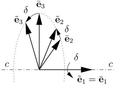
Rotation of  $\bar{\mathbf{e}}_i$  around  $\bar{\mathbf{e}}_1$  with the angle  $\delta$ , such that  $\tilde{\mathbf{e}}_2$  lies in the plane  $\mathcal{F}^*$ , and  $\tilde{\mathbf{e}}_3$  is directed normal to the plane  $\mathcal{F}^*$ . This yields the rotation tensor
