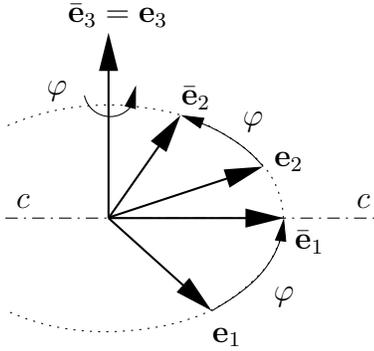
Rotation of  $\mathbf{e}_i$  in plane  $\mathcal{F}$  around  $\mathbf{e}_3$  with the angle  $\varphi$ , such that  $\bar{\mathbf{e}}_i$  is directed along the line  $c-c$ . This yields the rotation tensor
