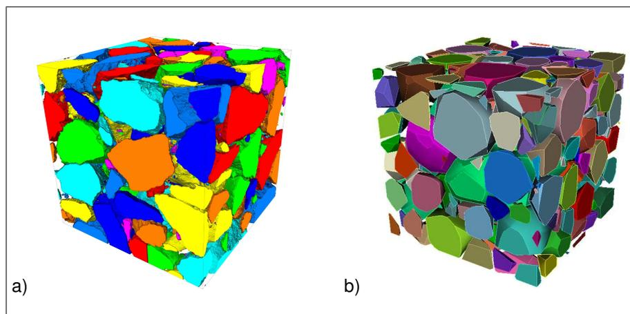
Figure 1: a)  $1000^3$  voxel cube reconstructed from XRCT data and b) artificial counterpart [2].
