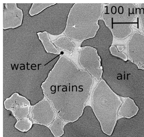
Figure 1: Reconstructed image of a partially saturated granular medium. Three phases can be observed: Water, air and solid grains.
