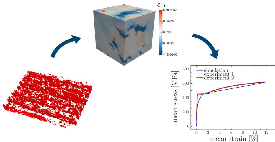
Figure 1: Simulation of flow curves based on 3D microstructures
