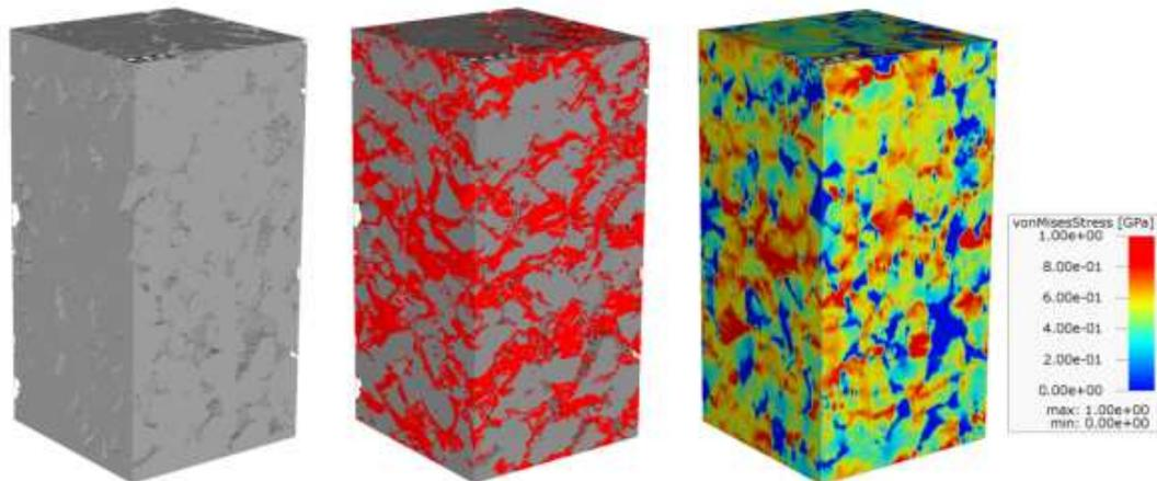
Figure 1: CT scan of Berea sandstone (left), damaged zones marked in red (middle), von Mises equivalent stress (right)
