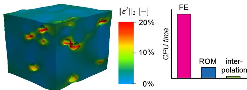
Figure 1: porous solid (*left*) and schematic comparison of the computational effort for the homogenized material response (*right*)
