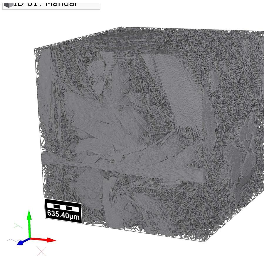
Figure 1: A volume element with aspect ratio of 150, volume fraction  $\phi = 20\%$  and isotropic fourth order fiber orientation tensor
