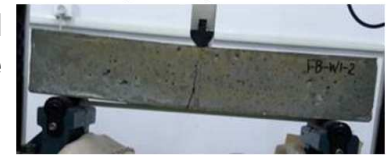
(b) failure pattern of FB-W1 concrete specimen
