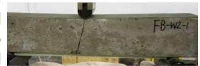
(c) failure pattern of FB-W2 concrete specimen J. Zhang; Z. Chen; X. Guo; W. Ma I J Mat Sci App 5(1):31-35, 2016
